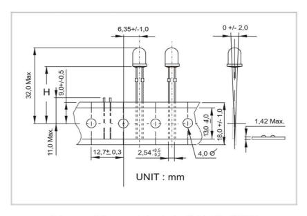
Unless specially requested, outgoing first lead is ANODE
